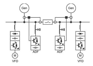
As can be seen, the setup is complex with multiple measurement points being tied to a summation transformer, and then the secondary of the summation transformer must be routed through all the ADF units. In the case of a bus tie or emergency generator setup, complexity increases further. A practical problem can be that the measurement resolution becomes poor due to the total equivalent CT ratio.
